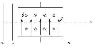
The slits define a beam of particles which passes straight through. Calculate the velocity of an undeflected electron in terms of the electric field E and the magnetic field B. If a voltage of  $100\,\mathrm{V}$  is applied to a  $1\,\mathrm{cm}$  deflection plate gap, what is the field required to let electrons of  $2\times10^7\,\mathrm{m/s}$  pass through.
